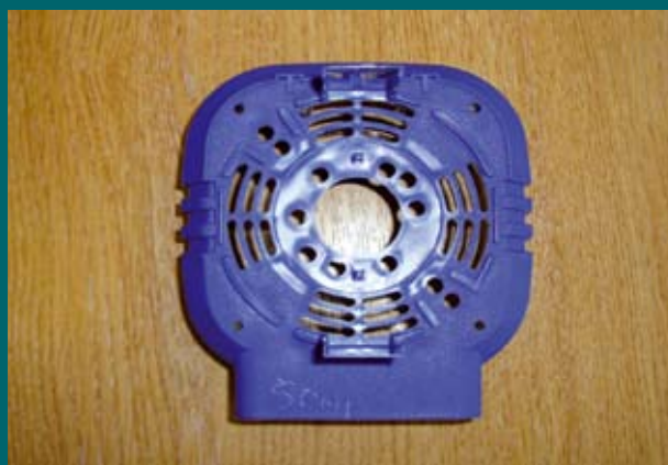
FIGURE 4: 92% FULLNESS (LEFT) WITH PIECE MISSING; 95% FULLNESS (RIGHT), THE SHAPE OF THE MOULDING COMPLETE
